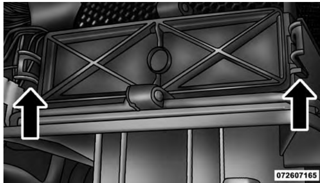
A/C Air Filter Replacement
