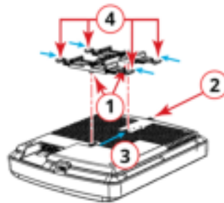
FIGURE 7 Attaching the T-bar Bracket to the AP
