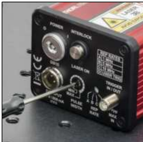
Figure 11 Use the included 2.5 mm flathead screwdriver to adjust the pulse width and repetition rate controls.
