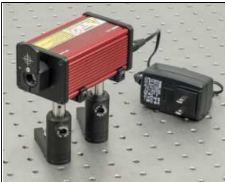
Figure 7 Laser Head Mounted Using the Included ECM225 Clamps
