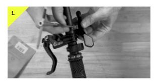
Position hinged clamp on bar and attach lever to clamp using one of the threaded hole options on lever body to achieve your desired position. Tighten with 3mm allen wrench to maximum 2nm. Note: This position can be changed after install to fine tune fit.
