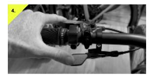
Push the lever 5-10 times to make sure the cable housing is fully seated and to check for play in the cable. Note: if there is play in the lever/cable, loosen cable fixing bolt with 3mm allen wrench and pull cable tight a second time. For micro adjustments, use the barrel adjuster on the lever where the cable enters.
