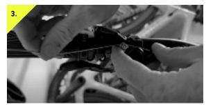
Pull cable taut and torque cable fixing bolt to 2.5 nm with a 3mm allen wrench. Note: Make sure cable is seated underneath the washer to ensure proper cable retention with the washer. At this point you may use a 2.5mm allen wrench to adjust the lever bottom-out position via the bolt located on the backside of the lever. Adjust based on personal preference.
