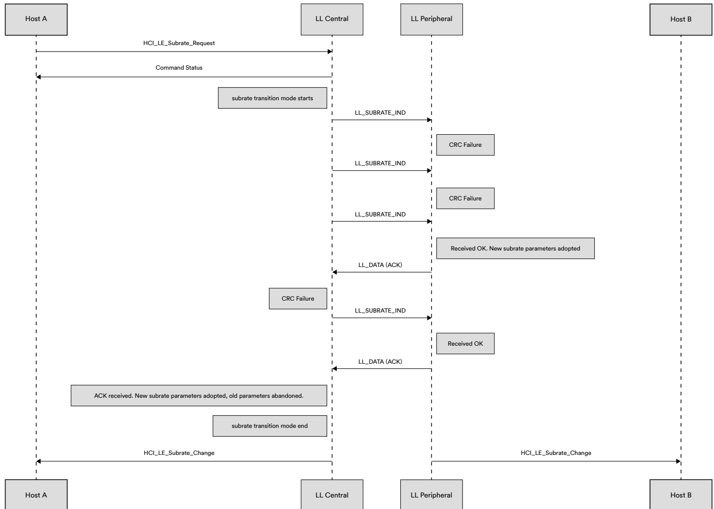
Figure 21 - Example subrate update procedure message sequence
