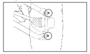
Recommended lubricant: Lithium-based grease
