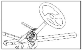
Lower universal joint, steering transmission shaft
