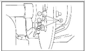
1. Brake pad wear indicator groove
