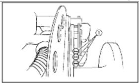
1. Brake pad wear indicator groove
