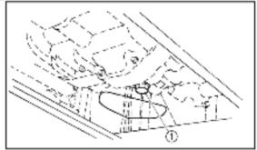
1. Engine oil drain bolt
