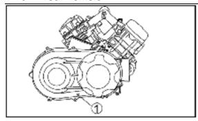
1. CVT Gear Box inspection hole
