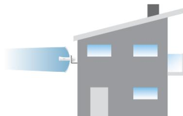
The PowerBeam mounted outdoors without the Reflector installed provides outdoor-to-indoor coverage using the 3 dBi Antenna Feed only.
