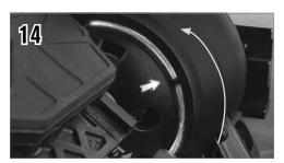
Line up the arrow on the dock with the alignment mark on the mount and press inward while turning the dock counterclockwise until the orange release button snaps into place in the hole on the dock.
