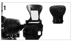
Remove the large cap covering the mirror on the front of the StarSense dock.
