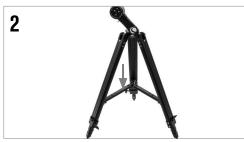
To set up the tripod, spread the legs outward until they are fully extended and push down the center leg
