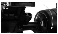
To remove the dock, press the orange release button and turn the dock clockwise until the bayonet mount
