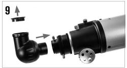
Locate the erect image diagonal and remove the plastic covers. Insert the barrel of the diagonal into the focuser and secure in place by tightening the set
