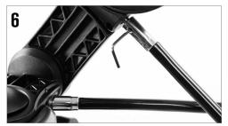
Place the slow-motion control knob over the D-shaped gear shaft and push inward to make sure it is fully seated. Use the hex key to tighten the setscrews onto the gear shaft. Return the hex key to its storage position in the front of the mount.
