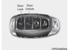
Press the button on the driver's outside door handle while carrying the Smart Key with you or press the Door Unlock button on the Smart Key, the driver's door will unlock.
