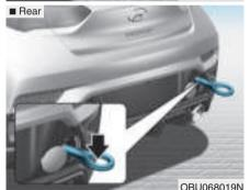
If towing is necessary, we recommend you have it done by an authorized HYUNDAI dealer or a commercial tow truck service. If a towing service is not available in an emergency, your vehicle may be temporarily towed using a cable or chain secured to the emergency towing hook at the front (or rear) of the vehicle.
