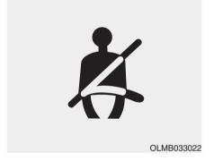
As a reminder to the driver, the seat belt warning light will illuminate for approximately 6 seconds each time you place the ignition switch to the ON position regardless of belt fastening. At this time, if the seat belt is not fastened a warning chime will sound for 6 seconds.
