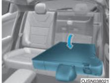
3. Remove the belt from the clip (1) and pull up the seatback folding lever (2), then fold the seat toward the front of the vehicle.
