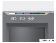
The number of LEDs illuminated indicates the relevant engine speed Different colored LEDs will be illuminated as engine speed nears the maximum allowed speed.
