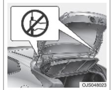
Do not hold on to or try to pull on the liftgate strut. Be aware that the deformation of the liftgate strut may cause vehicle damage and risk of injury.
