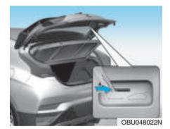
Your vehicle is equipped with an emergency liftgate safety release lever located on the bottom of the liftgate inside the vehicle.
