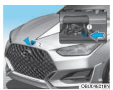
3. Go to the front of the vehicle, raise the hood slightly, push up the secondary latch (1) inside of the hood center and lift the hood (2).
