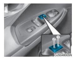
The driver side door armrest is equipped with a central door lock switch. The lock button is indicated by a (☆) symbol. The unlock button is indicated by a (☆) symbol.
