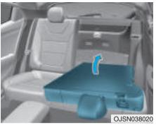
4. To use the rear seat, lift and unfold the seatback to the upright position. Push the seatback firmly until it clicks into place. Make sure the seatback is locked in place.
