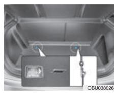
First secure the child restraint with the LATCH lower anchors or the seat belt. If the child restraint manufacturer recommends that the top tether strap be attached, attach and tighten the top tether strap to the top tether strap anchor.
