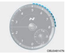
The yellow and red LEDs show the range of recommended engine operation speed. As the engine oil temperature warms up, the recommended engine speed range also extends. Avoid driving with engine speeds in the yellow and red warning fields. In particular, do not drive with the engine speed in the red warning field.
