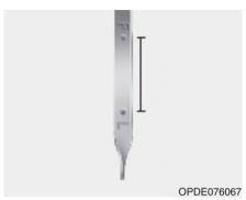
Pull the dipstick out again and check the level. The level should be between F and I
