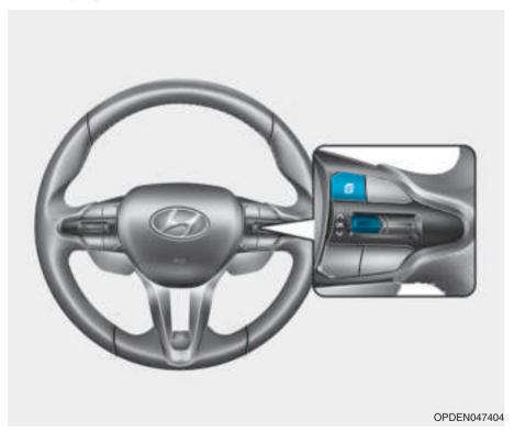
The LCD display modes can be changed by using the control buttons.
