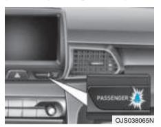
As a reminder to the front passenger, the front passenger's seat belt warning lights will illuminate for approximately 6 seconds each time you place the ignition switch to the ON position regardless of belt fastening. If you continue not to fasten the seat belt and you drive over 6 mph (9 km/h), the warning light will stay illuminated
