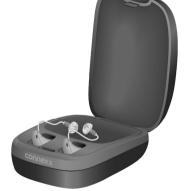
repeated every 20 minutes. Depending on the usage of your hearing instruments, you have approximately 1.5 hours to charge your hearing instruments before they stop working.
