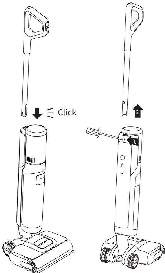
**Note:** To disassemble, extend a hard object into the hole of the appliance as indicated to press in the contacts and pull the handle upwards at the same time.
