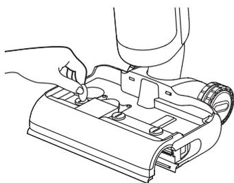
5. Wipe the suction inlet with a dry cloth or wet tissue. Do not rinse the brush assembly with water.
