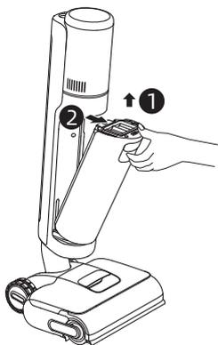
2. Remove the filter from the used water tank cover. Pull up the used water tank cover and pour out the sewage.
