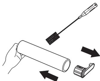
4. Use a coin to turn the locking knobs on the roller brush cover to remove the cover.
