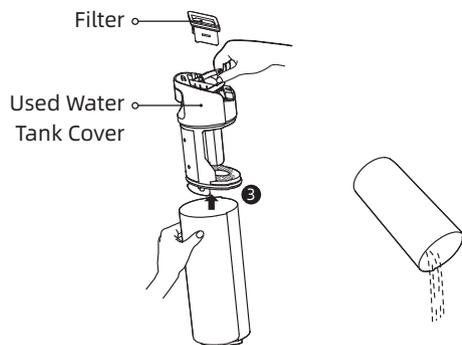
3. Rinse the used water tank and tank cover with water. Use the provided cleaning brush to clean the inner wall of the tank.
