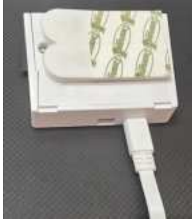
Figure 3: USB-C Cable plugged into SAFEST Activity Sensor
