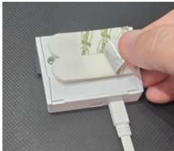
Figure 4: Peel off both adhesive backing strips
