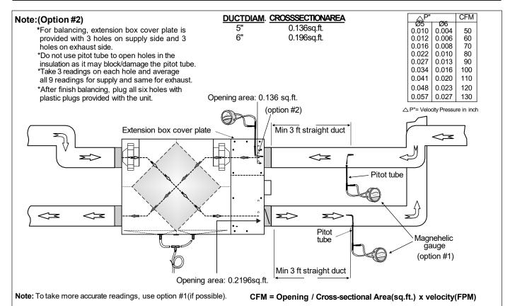
The accuracy of the flow reading will be affected by how close to any elbows or bends the readings are taken. Accuracy can be increased by taking an average of multiple readings as outlined in the literature with the Pitot tube.
