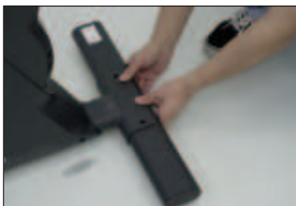
9. Align the holes on #3 rear stabilizer and the rear bracket on the #1 main frame.
