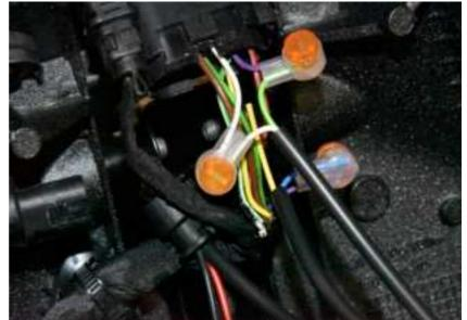
Connect the EWA Yellow wire to the White wire end, which is at the wiring harness side. Use a yellow butt connector.
