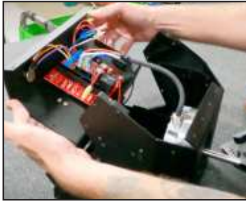
Lift out circuit board panel.
