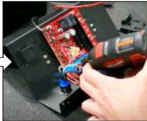
Loosen circuit wire screws using a flat head drill bit, pull out wires from bottom slots.
