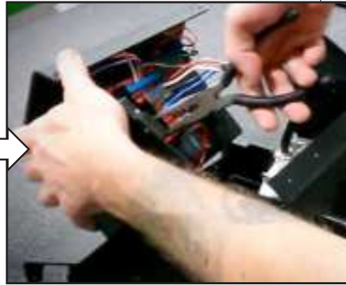
Remove Circuit board connectors using needle nose pliers.
