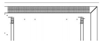
3. Attach the wall bracket lock piece onto the bracket with screws and slide the lock piece into the locking slot on the back of the heater. Tighten the screws:
