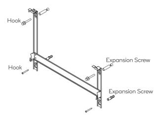
2. Align the 4 holes in the back of the heater with the 4 hooks on the wall bracket and push it on, then slide them into the slots to click on:
