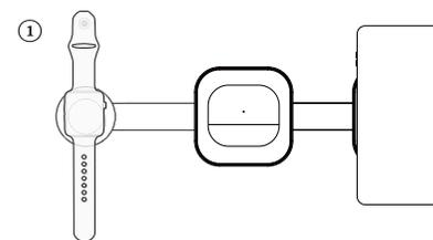
Place the device flat on the charging pad, making sure it is properly centered, then initiate charging.
