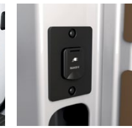
Available 120-volt outlet is easily accessible when you're outside.
