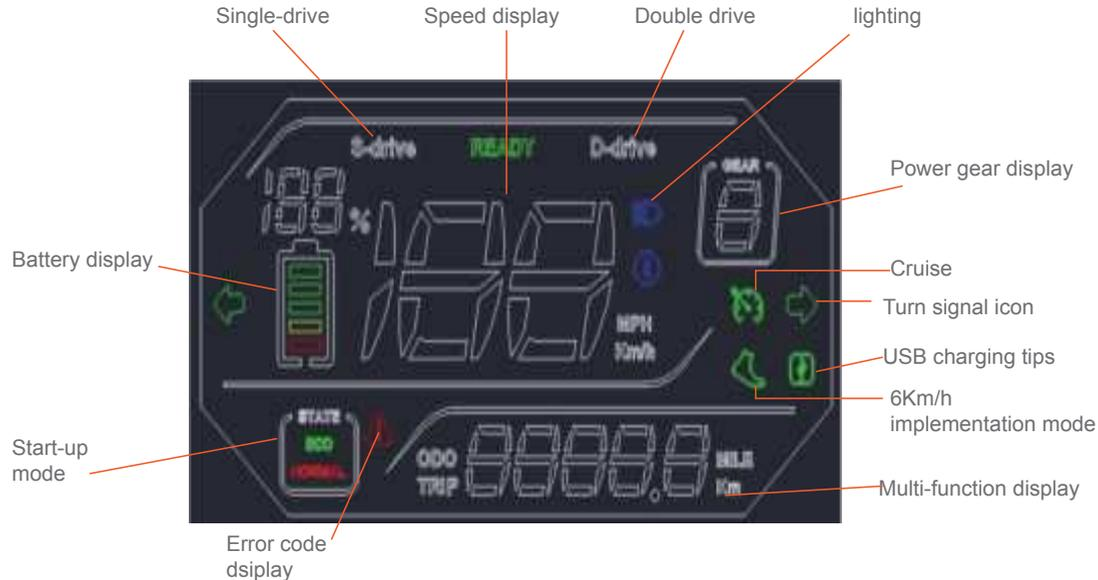
E-01:Rear-drive Hall failure, E-11:Front-drive Hall failure
