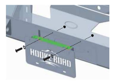
Secure the bumper to the vehicle frame.
