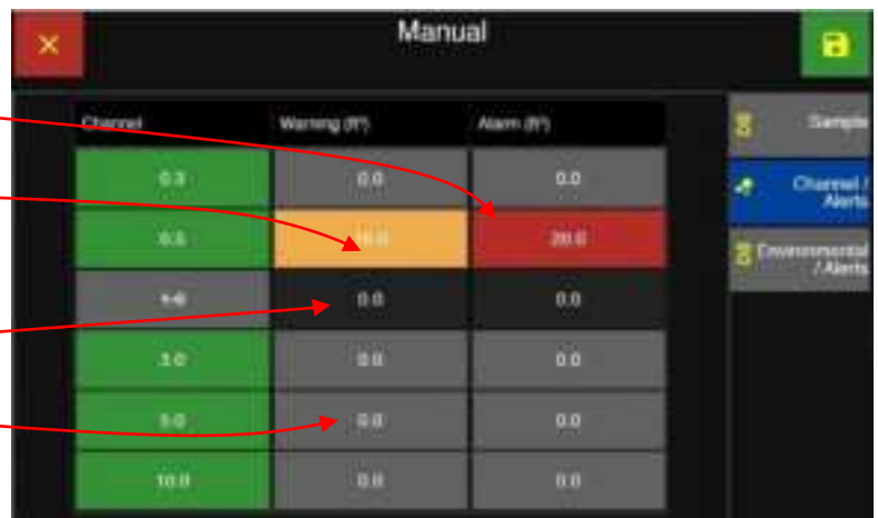
Manual Sample Plan: Channel, Warning and Alarms
