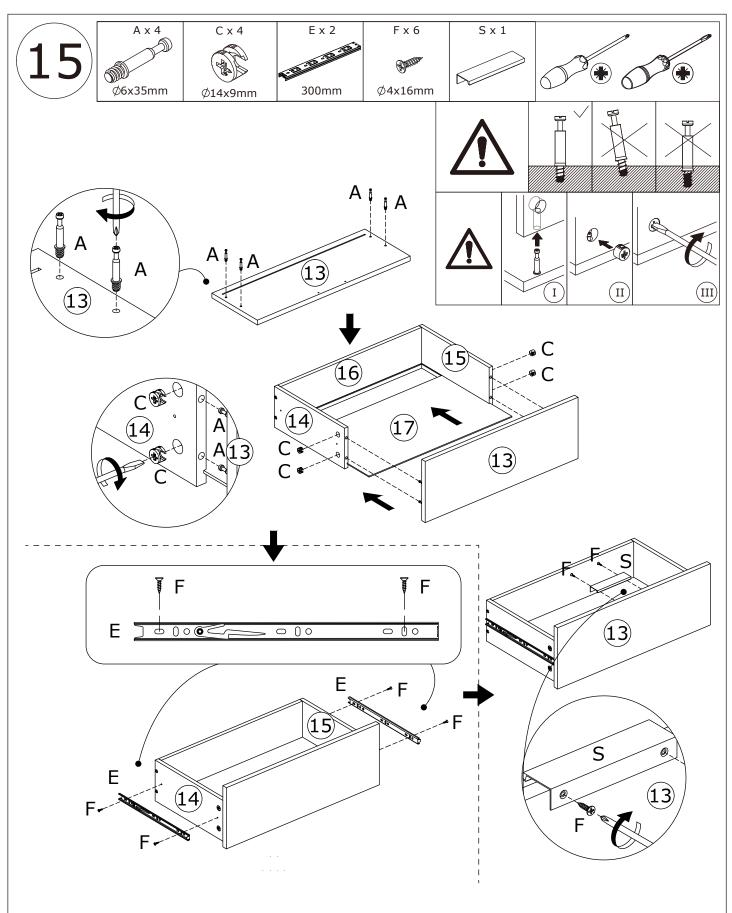
Insert quickfit screw(A) into plate 13 as shown. Slide plate 17 along grooves, then attach plate 13,put cam lock(B) into holes in plate 14,15 and turn clockwise to tighten as shown. Fix runner(E) to plate 14 and 15 using screw(F) as shown. Fix handle(S) to drawer face plate using screw(F) as shown.
