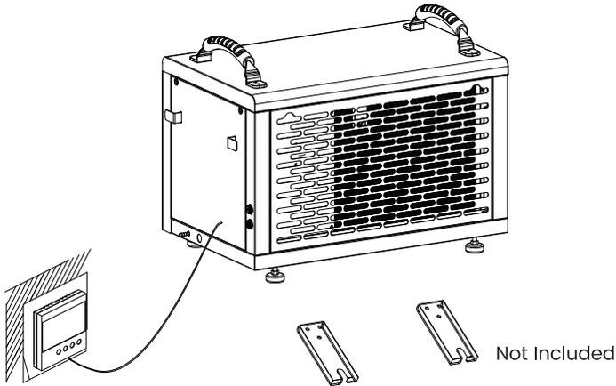
Remove the original leveling feet and attach the gaskets included in the CPG130A package for ceiling mount installation.
