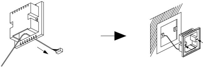
3. Attach the XH Connector to the corresponding port on the back of the remote controller. Next, reattach the mounting bracket to the controller interface. Align the clasps with the slots, press firmly, and they will click into place.
