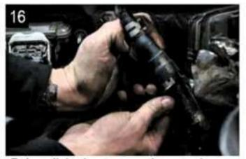
Reinstall the heater core hose to the steel hose bib.
