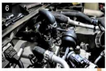
Remove the coolant hose from the EGR cooler going to the coolant tank.
