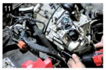
Remove the 3 8MM bolts holding the wiring to the cooler.
