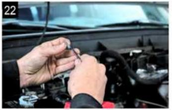
Cap the factory vacuum line with provided vacuum cap.
