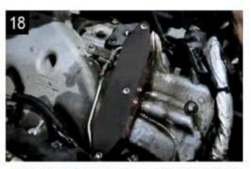
Install the Coolant cover plate with 3pcs socket head bolts provided.
