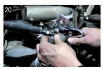
Cut the "T" out of the factory coolant hose. (This hose had the branch going to the EGR)
