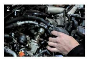
Now Remove the EGR cooler outlet to Intake tube.
