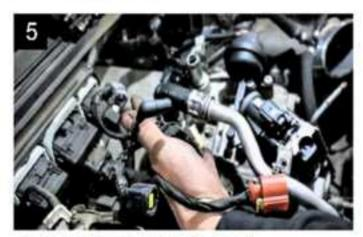
Remove the EGR motor, and temperature sensor plugs along with the one vacuum line.
