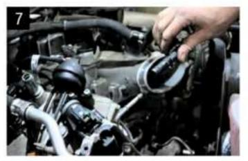
Remove the 3/8" coolant line from the cooler. This will be cut and reconnected later.
