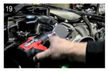
Install the Intake plate with 2pcs socket head bolts.
