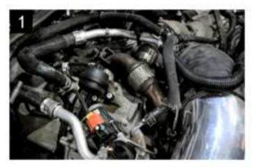
Start by unplugging the batteries. Then remove the exhaust manifold to EGR cooler inlet tube. There are two bolts on each flange and one on a retainer bracket.
