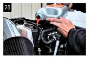
Refill coolant, Reconnect batteries and start the truck to check for leaks.
