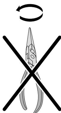
**EN** Rotation in counter-clockwise direction will destroy the adapter and its built-in electronic components.
