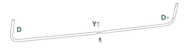
(4). Connect #D (Left Bottom Support) and #D-1 (Right Bottom Support) to #B (Back Leg) with four sets of #N (M6x95 Bolt Set).
