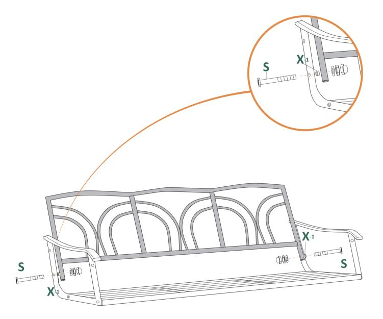
(3). Connect **#G** (Swing Arm), **#J** (Back Conecting Bar), **#H** (Backrest) with **#V** (M8x90 Bolt Set) and **#X-1** (Spacer).
