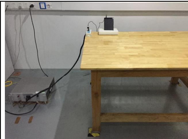
Conducted Emissions Test Setup Front View
