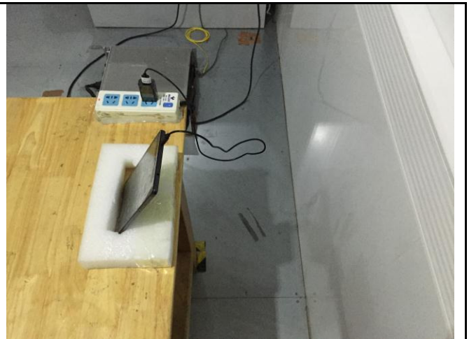
Conducted Emissions Test Setup Side View
