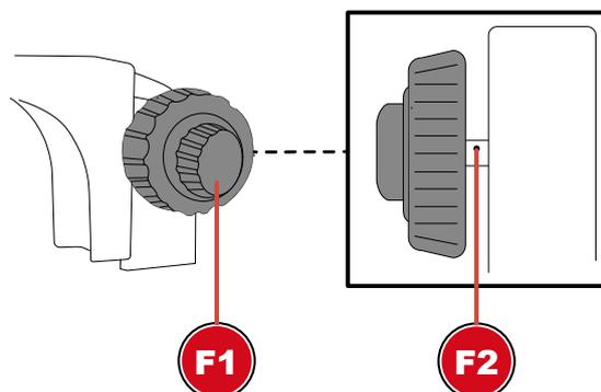
*Illustration 2: Friction adjustment on the focus wheel (left or right, depending on model).*
