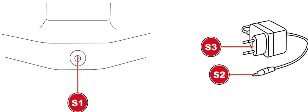
S1 Connection socket for DC barrel connector
