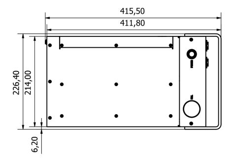
General tolerance: ± 0,25mm Dimension in millimeter
