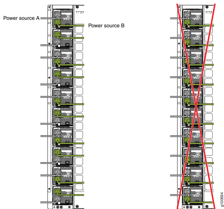
Figure 121: Proper Load Balancing for QFX10000-PWR-AC Power Cables on QFX10016
