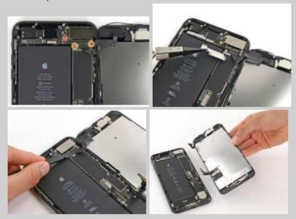
7. Remove the four Y000 screws securing the bracket over the home/Touch ID sensor Remove the bracket that secures the home/Touch ID sensor.
