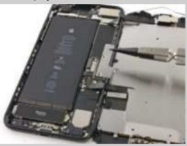
5. Use the point of a spudger to lift the battery connector out of its socket on the logic board. Use the flat end of a spudger or a fingernail to disconnect the two lower display connectors by prying them straight up from their sockets on the logic board.
