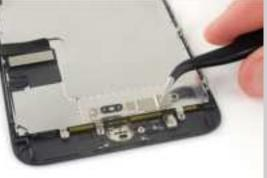
8. Pry under the left edge of the home button cable connector to disconnect it from its socket. Carefully pry up the underlying connector and move it out of the way of the home/Touch ID cable. If the connector doesn't pry up easily, use a hair dryer to heat and soften the adhesive securing the connector, and then try again.
