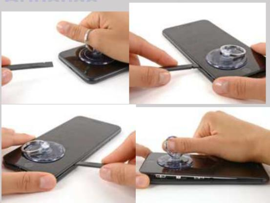
3. Slide an opening pick underneath the display along the top edge of the phone to loosen the last of the adhesive. Pull the display assembly slightly away from the top edge of the phone to disengage the clips holding it to the rear case. Open the iPhone by swinging the display up from the left side, like the back cover of a book.
