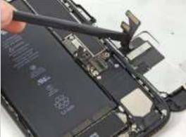
6. Remove the three tri-point Y000 screws securing the bracket over the front panel sensor assembly connector. Remove the three tri-point Y000 screws securing the
