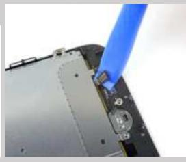
Use an opening pick to gently separate the adhesive holding the home/Touch ID sensor cable to the back side of the display panel. Remove the home/Touch ID sensor assembly.
