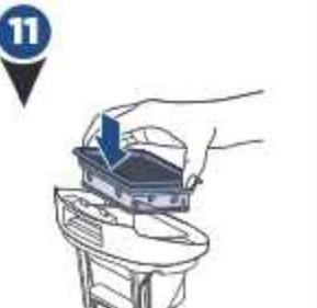
Place vacuum filter back into the top of the dirty water tank.
