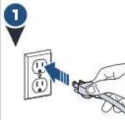
Plug machine into a properly grounded outlet.
