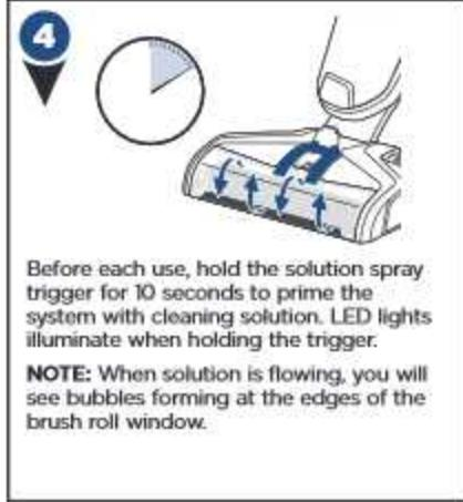
Before each use, hold the solution spray trigger for 10 seconds to prime the system with cleaning solution. LED lights illuminate when holding the trigger.
