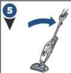
Recline the machine while in storage tray. Allow the machine to run for 10-15 seconds until all water is picked up. Repeat as needed.
