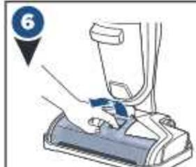
Grasp brush roll window at the front of the window and pull upward to remove.
