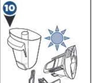
Leave parts out to dry before reassembling.
