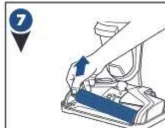
Pull brush roll out by grabbing the brush roll tab and pulling upward.
