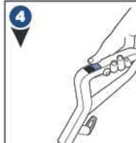
Turn the machine ON by pressing the Hard Floor button.
