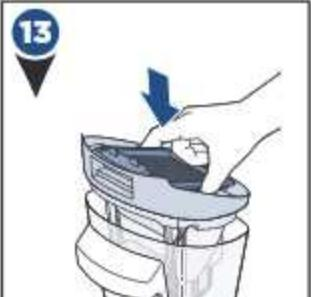
Once parts are dry, reassemble and replace the top of dirty water tank.
