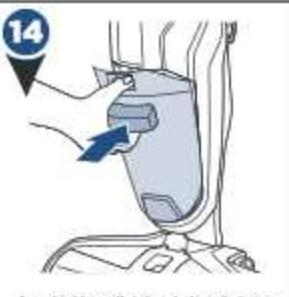
Angle the dirt tank back into body of machine inserting bottom first. Then tilt the top of the dirt tank toward the machine and push into place until you hear a click.
