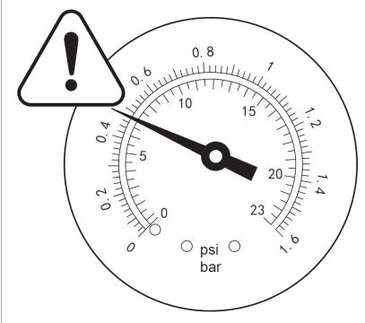
**NOTE:** The pressure gauge is for maintenance purposes only, and the pressure gauge value is just for reference. It should not be used as a precision instrument.
