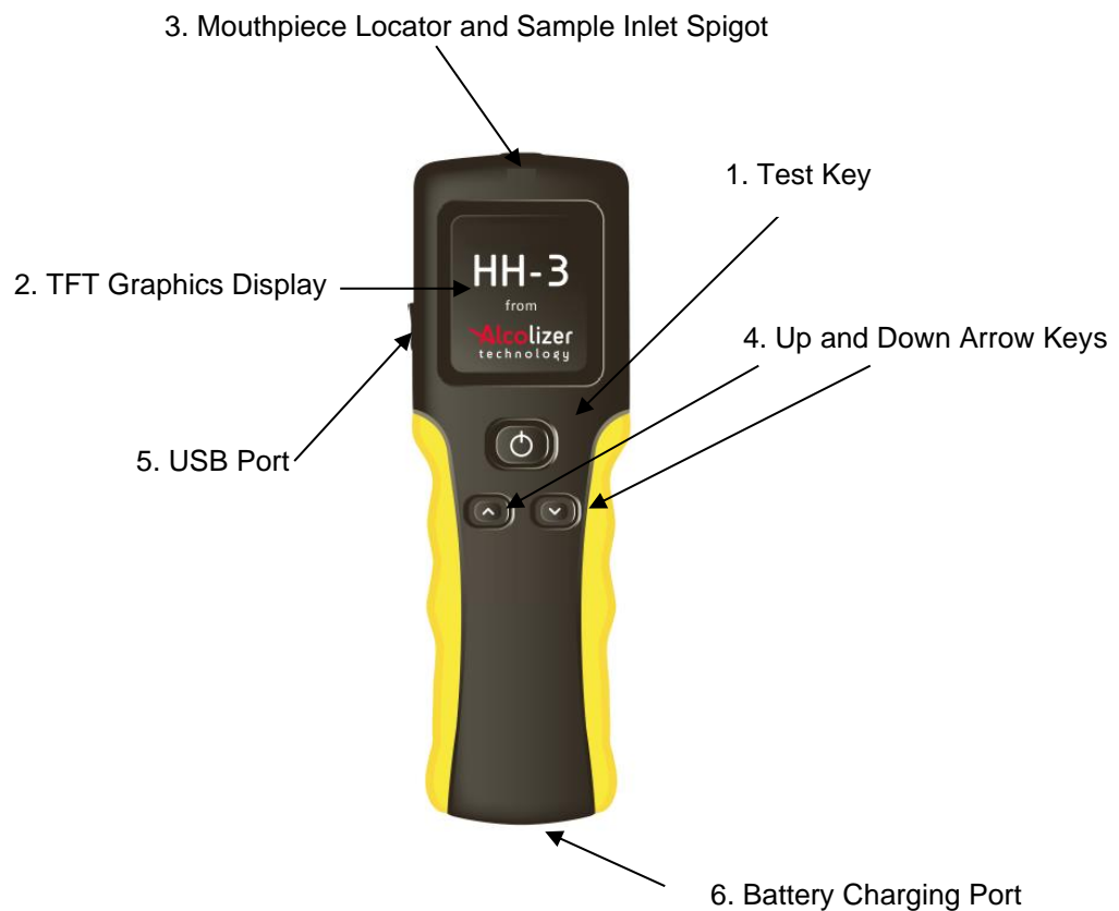
Figure 1 - User Display, Buttons and Adapter Sockets
