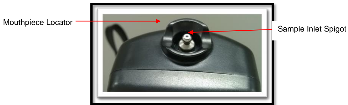
Figure 2 - Mouthpiece locator and Sample inlet spigot
