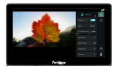
In Monitor Functions > Focus > Peaking, after activating peaking, the image will be highlighted to show focus areas. Choose a highlight color suitable for the current shooting environment. Adjust the sensitivity to increase or decrease the highlighted area, then adjust the focus in real-time by moving the focus ring until the desired focus area is clearly marked
