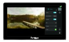
Monitoring Normal Exposure: in the area options, select "Medium" and set the IRE threshold between 40-70. A new Range option will appear, allowing more precise control of the zebra lines in the image to achieve optimal results.
