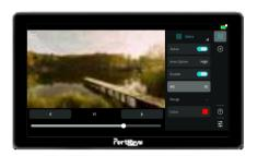
Monitoring Overexposure: select "High" in the area options and set the IRE threshold between set the IRE threshold between 80 and 90 to prevent overexposure. Depending on your shooting needs, use zebra to monitor and mark exposure thresholds, adjusting the camera settings based on the feedback from the image.
