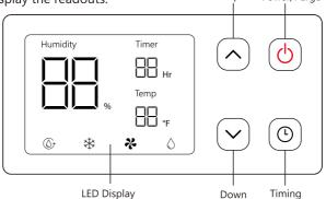
🗒 is humidity percentage value. If no operations on the control panel, this number is the humidity readout of the inlet air the dehumidifier detects which is similar to the current room humidity level. When you are pressing the 🔊 or 👽 button to set the target humidity percentage value, this digital number will turn to display the previous setting value and keep blinking.
