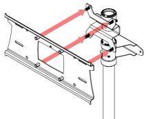
Fix the PZX back plate to the PS3U1 mount adapter using the 4 x M10 x 25 screws. Cables are fed through central aperture in back plate.
