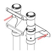
Decide where the product is to be installed. Measure 102.5mm out from wall (not skirting) mark, drill and secure the floor plate into position. (Fixings not supplied).
