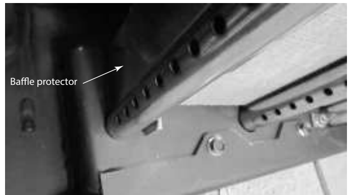
Figure 4.9 Reinstall Baffle Protection Channel
