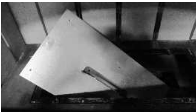
Figure 4.12 Removal of Combustion Cover
