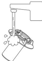
3 Insert the Waste Filter back into the Water Station, tighten the knob, put the cover back, and place the Water Station at its original position.
