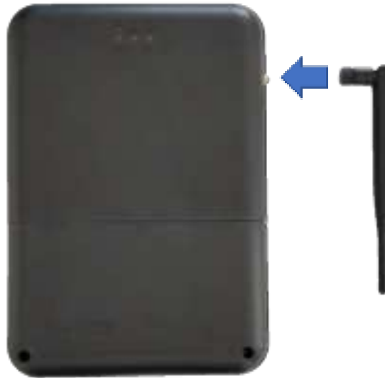
Illustration 11 : Antenna location to Combox
