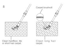
Note: what is the rolling brush blocking protection? During the operation of the electric floorhead, if there is a large volume of foreign matter inhaled or too much fiber wound, or even a child in the play of the machine mistakenly put his hand into the nozzle, resulting in the brushroll abnormal stop, the electric floorhead will stop working, in order to protect personal safety and brush motor.
