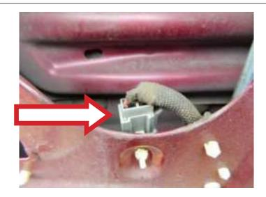
**STEP 3a:** Attach the window lift motor connector to the door.
