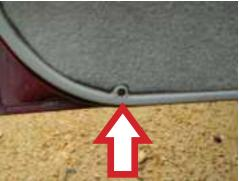
**STEP 2:** Using a trim panel removal tool, remove the door handle trim bezel.
