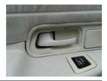
**STEP 10:** Verify that the door trim panel is tight and that the window glass is operating smoothly. If necessary, use a silicone spray lubricant in the door glass channel.
