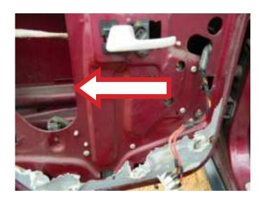
**STEP 2:** Using a rivet gun and rivets, attach the window regulator to the door.
