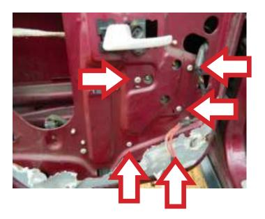
**STEP 9a:** Drill out the remaining body of the rivet with an 1/8" drill bit. **NOTE:** BE SURE TO HOLD THE DRILL BIT STRAIGHT. YOU DO NOT WANT TO MAKE THE HOLES IN THE DOOR OBLONG.
