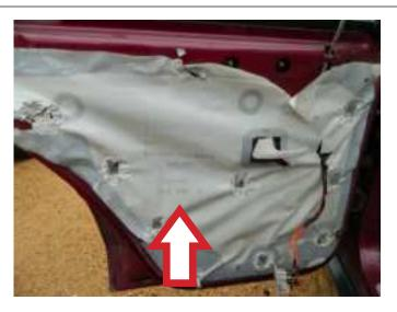
**STEP 6:** Using a trim panel removal tool or the flat side of a tool handle, press the window lift motor connector into the door. **NOTE:** Do not disconnect at this time.
