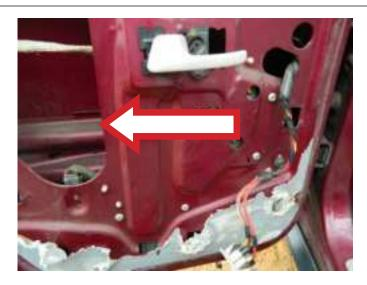
**STEP 11:** Remove the three (3) window lift motor attaching screws. **NOTE:** Some of the window lift motors were attached with a Phillips head screw, while others were attached with a T-25 Torx bit. You can tell this by looking at the bolts through the hardware access screws.
