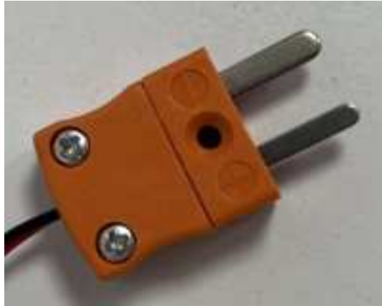
Figure 3 Thermocouple end of Element-B connection cable
