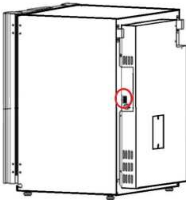
Figure 1 Remote Contact panel on the back right side of a Sanyo/PHCBI MCO-18AC incubator
