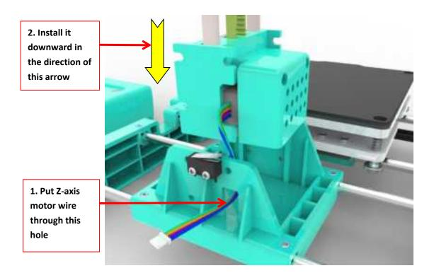
2. After insert the XZ Axis, Fixed with 2 screws.
