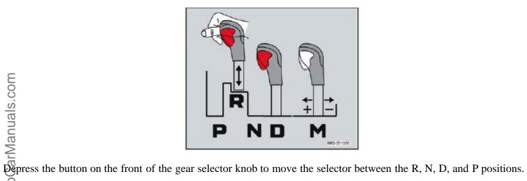
The gear selector can be moved freely between the Geartronic (manual shifting) and Drive (**D**) positions while driving.
