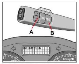
Controls on the left-side steering wheel lever
