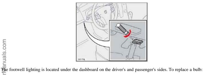
Insert a screwdriver under the edge of the lens. Turn the screwdriver gently to detach the lens.
