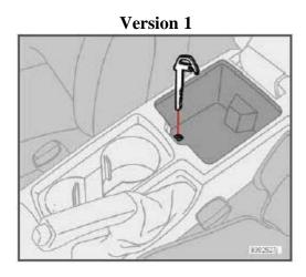
If necessary, the trunk can be opened mechanically using the key blade. Depending on the model, the keyhole may be found in different places.
