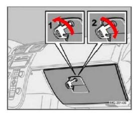
The glove compartment can only be locked and unlocked using the detachable key blade on the remote control. See page 111 for information on removing the key blade from the remote control.
