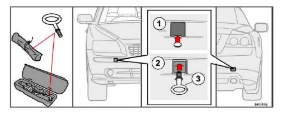
The towing eyelet is located under the floor of the cargo area with the optional temporary spare tire or in the bag stowed in the ski hatch. This eyelet must be screwed into the positions provided on the right sides of either the front or rear bumper (see illustrations).
