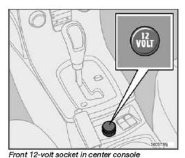
The 12-volt socket can be used to plug in certain accessories such as cellular telephones, etc. The key must be in position I (or higher) for the auxiliary socket to function.
