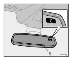
The compass may need to be calibrated in certain cases. If calibration is required, the character C appears in the mirror's display.
