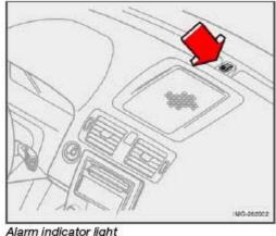
The status of the alarm system is indicated by the indicator light on at the top of the dashboard (see illustration):
