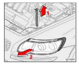
The entire headlight housing must be lifted out when replacing the high/low beam, parking light, turn signal, and side marker bulbs. To lift out the housing:
