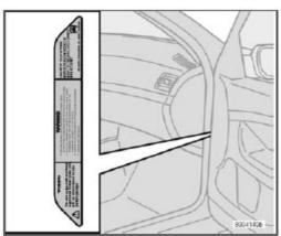
Airbag decal in the front passenger's door open-
