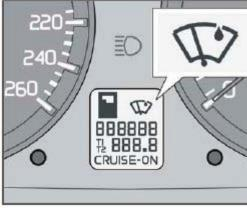
The rain sensor automatically regulates windshield wiper speed according to the amount of water on the windshield. The sensitivity of the rain sensor is adjusted by moving the thumb wheel (C in the illustration on the previous page) up (the wipers will sweep the windshield more frequently) or down (the wipers will sweep the windshield less frequently).
