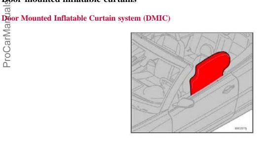
The DMIC is a supplement to the structural side impact protection. These inflatable curtains are concealed in the upper section of the driver and passenger doors.
