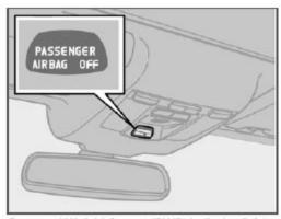
Occupant Weight Sensor (OWS) indicator light
