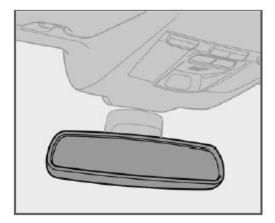
Auto-dim function An optional integrated sensor reacts to headlights from following traffic and automatically reduces glare.
