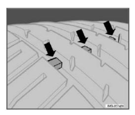
The tires have wear indicator strips running across or parallel to the tread. The letters TWI are printed on the side of the tire. When approximately 1/16" (1.6 mm) is left on the tread, these strips become visible and indicate that the tire should be replaced. Tires with less than 1/16" (1.6 mm) tread offer very poor traction.
