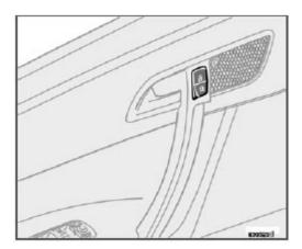
The switches near the door opening handles on the driver's and passenger's doors can be used to lock or unlock both doors and the trunk, and to set the alarm.
