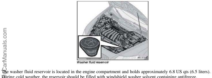
During cold weather, the reservoir should be filled with windshield washer solvent containing antifreeze.
