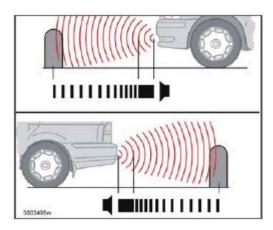
The park assist system(s) are designed to assist you when driving into parking spaces, garages, etc. They utilize ultrasound sensors located in the bumpers to measure the distance to a vehicle or other object, or a person who may be close to the front or rear of the vehicle.
