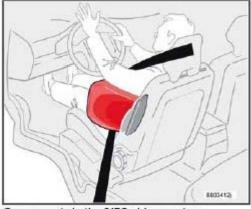
Components in the SIPS airbag system
