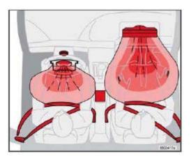
The front airbags supplement the three-point seat belts. For these airbags to provide the protection intended, seat belts must be worn at all times.
