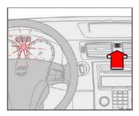
The four-way flasher should be used to indicate that the vehicle has become a traffic hazard. To activate the flashers, press the triangular button in the center dash. Press the button again to turn off the flashers.
