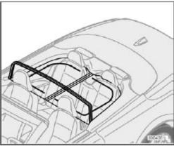
Wind blocker (retailer installed accessory)
