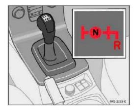
Reverse gear should only be engaged from a complete stop.
