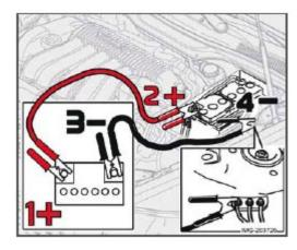
Follow these instructions to jump start your vehicle's dead battery or to jump start another vehicle's dead battery using your vehicle. If the 12-volt auxiliary battery to be used is in another vehicle, check that the vehicles are not touching to prevent premature completion of a circuit. Be sure to follow jump starting instructions provided for the other vehicle.
