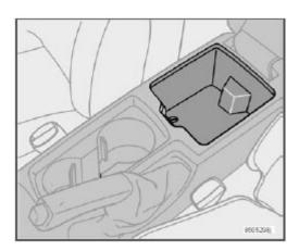
This compartment can be opened by pressing the front edge of the button.
