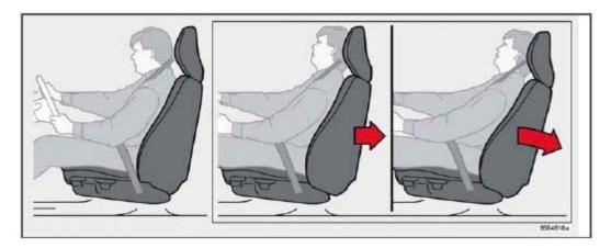
The WHIPS system consists of specially designed hinges and brackets on the front seat backrests designed to help
