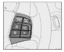
The four buttons on the steering wheel keypad can be used to control the audio system.
