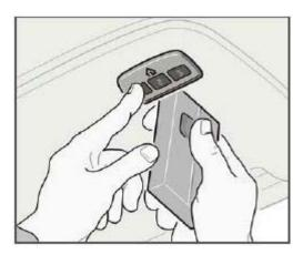
HomeLink<sup>1</sup> is a system that can be programmed to learn the codes of three different remote controlled-devices (for example, a garage door opener, remote lighting, entry gate). HomeLink's sun visor-mounted transceiver, powered by your car's electrical system, may then be used in place of your handheld remote controls. The HomeLink transceiver consists of three programmable buttons and an indicator light.
