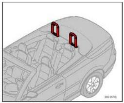
Deployed ROPS roll bars
