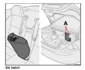
The center section of the rear seat backrest can be opened to create space for carrying long, light objects (max. length 6.5 ft/2 meters, max. weight 55 lbs/25 kg). To do so, the center section (cushion) of the rear seat backrest must be removed, the tire repair kit (if the vehicle is so equipped) must be removed and stowed in the trunk, and the plastic hatch in the trunk must be opened.
