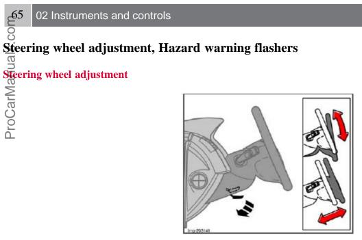
Both the height and the reach of the steering wheel can be adjusted to a comfortable position for the driver.
