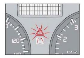
If the vehicle has been involved in a collision, the text CRASH MODE SEE MANUAL may appear in the information display. This indicates that the vehicle's functionality has been reduced.
