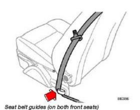
These guides are designed to help provide easier access to the seat belts. A belt can be taken out of the guide and slid to the rearmost part of the lower seat belt anchorage rod to make it easier for passengers to enter or exit the rear seat.
