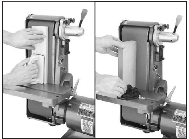
Figure 40. Examples of vertical face and edge sanding.
