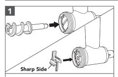
Insert the Grind Screw into the Main Housing securely. Place the Blade over the end of the Grind Screw.
