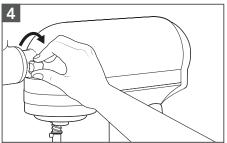
Tighten the Stand Mixer attachment hub knob until the attachment is completely secured to the Stand Mixer.
