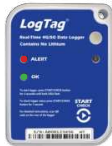
Figure 2: Green and Red LEDs flash in sequence.
