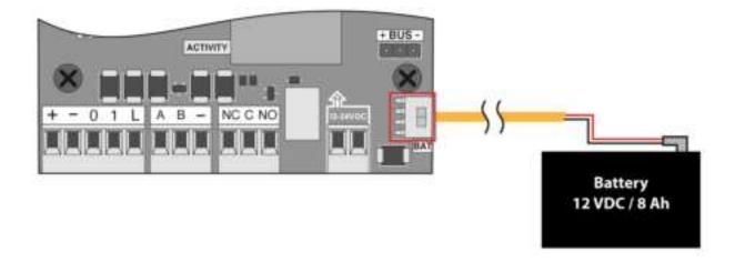
The onboard power supply is a 12.0V 5A 60-watt, class-2 power supply. This connection is polarity sensitive, meaning that it has fixed positive and negative connections. From the onboard power supply, connect a red 18/2 wire from the positive (+) DC terminal to the positive (+) Cloud Node connector. Connect a black 18/2 wire from the onboard power supply negative (-) DC terminal to the negative (-) Cloud Node connector (A/1 in the illustrations above).
