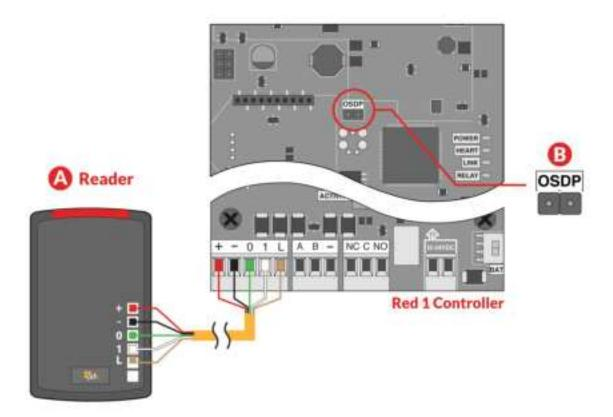
(A) Main Reader - The main reader is mounted at the door with a 22/5 or 22/6 wire ran to the door controller. Wire the reader to the controller as shown above. Be sure to check polarity and voltage prior to powering the controller.
