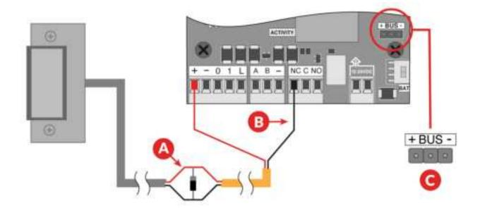
(A) Diode: The provided diode MUST be installed when using a strike. Install at the strike with the stripe of the diode on positive (+) and the black on negative (-).
