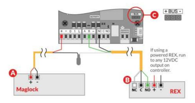
**NOTE**: For UL-certified wire installations, all wire running from a door controller to a lock, strike, or reader device must be less than 98.5 feet (30 meters).
