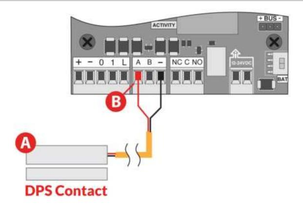
(A) DPS: The Door Position Sensor is mounted on the door frame in the desired location with a 22/2 wire running from the DPS to the controller. (When using two DPS sensors for double doors, wire them in series with only two conductors running back to the controller.)
